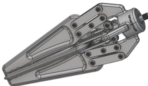
**Figure 1:** CAD model representation of a gripper (Pérez, 2016)
