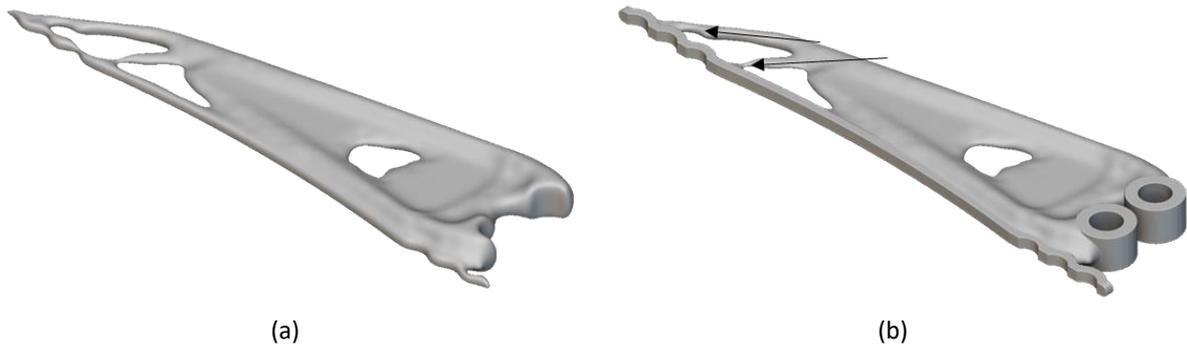
**Figure 4:** (a) Result of the surface smoothing; (b) Smoothen surface with the updated holes and gripping faces.
