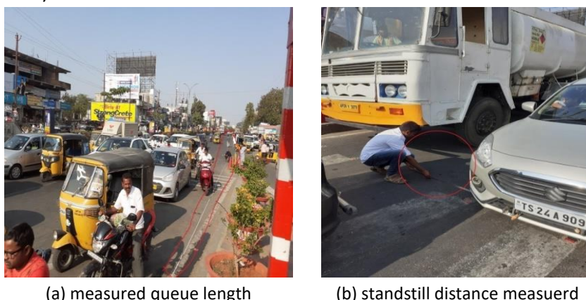
Figure 9: Measured (a) Queue Length, and (b) Standstill Distance of Selected Approaches of Intersections
