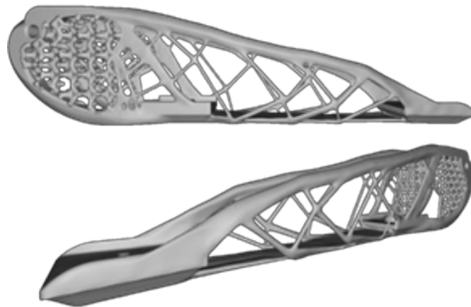
Figure 11: GD_BC_RP With Lattices Added in nTopology.
