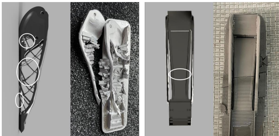
Figure 13: CAD Model With the Areas to Rework Marked and Falling Printed Parts.
