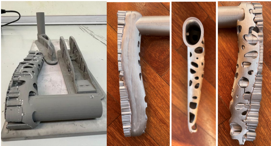
Figure 13: Influence of Component Positioning in the Sintering Plate: Lattice Optimized Door Handle
