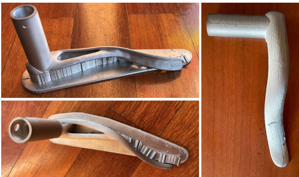
Figure 14: Door Handle After Sintering and the Effect of Support Collapse
