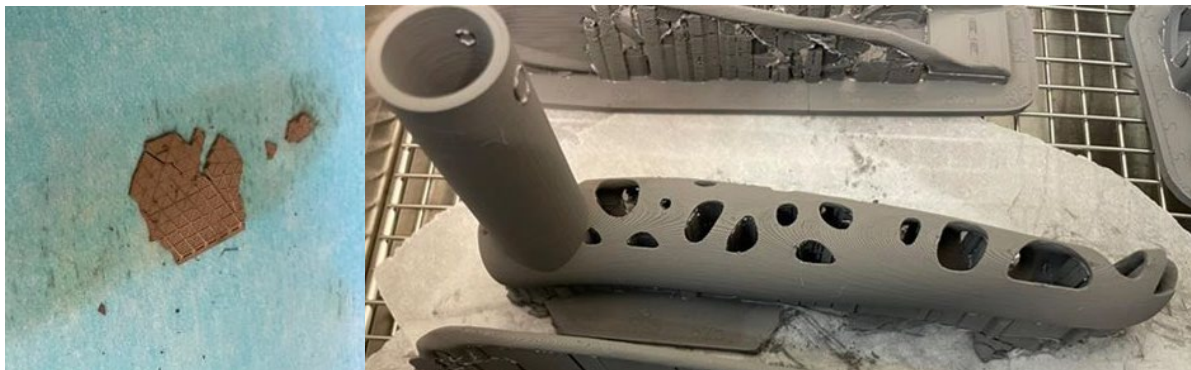
Figure 12: Material Loss During Printing and Subsequent Interference in Debinding Step
