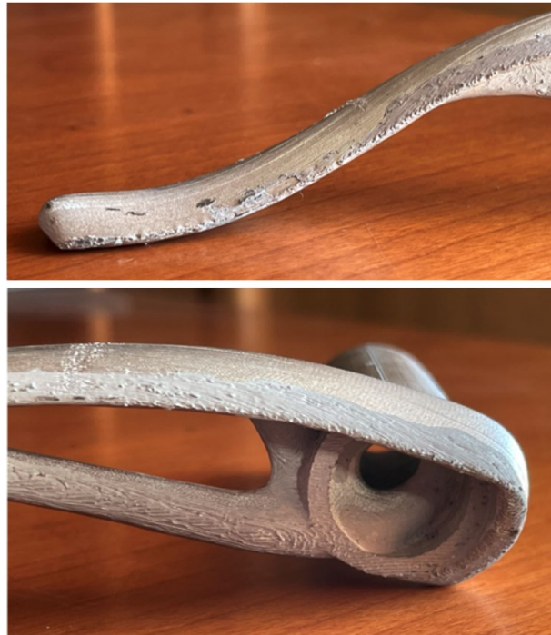
Figure 15: Roughness at the Interface Between Supports and Component
