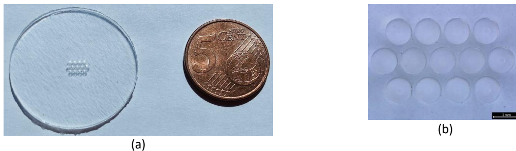
Figure 4: Microlens array produced using the EDM mould insert (a) and DM image of lens array produced with \mu -EDM mould insert (b) Scale bar is 3 mm
