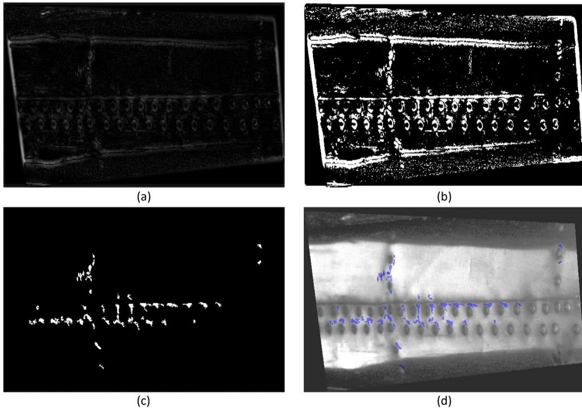
**Figure 12:** The steps of automated quantification of hidden corrosion spots on a D-Sight image: determination of the  $\Delta E^*$  local metric (a), quantization using Otsu's method (b), application of morphological operations (c), visualizing the mask of quantified hidden corrosion on the pre-processed D-Sight image (d) (Katunin et al. 2023)
