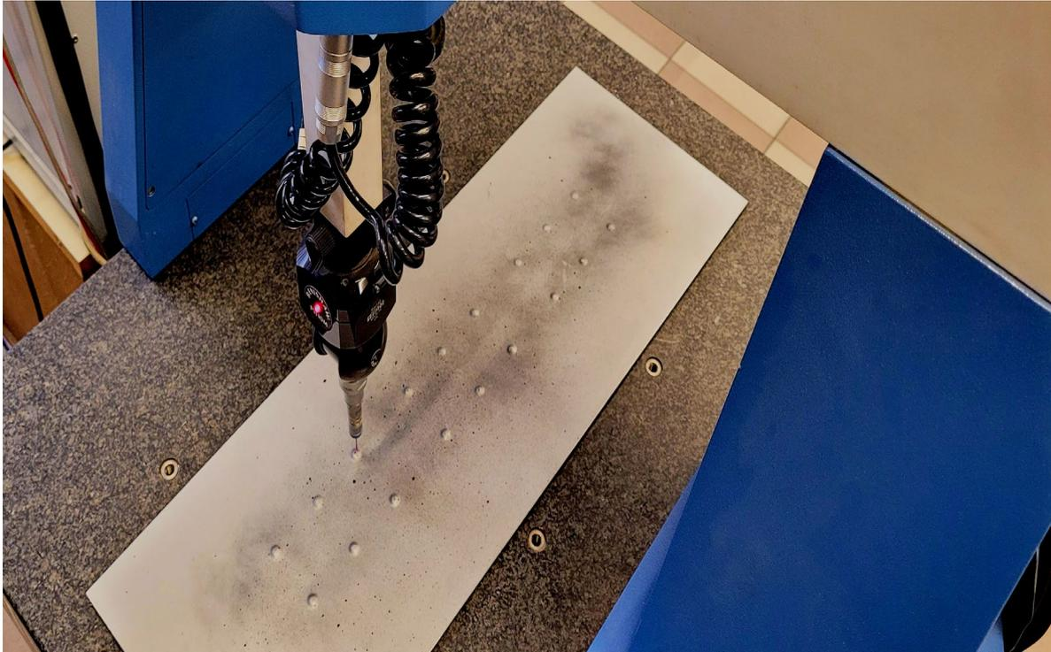
**Figure 10:** The process of measuring deformation heights using the coordinate measurement machine
