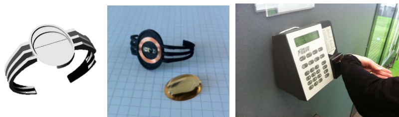
Fig. 9. 3D model, quick prototype and operational testing of the access control bracelet.
